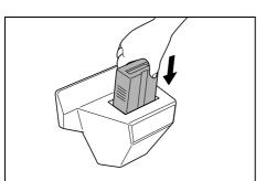
Insert the key counter securely into the key counter slot.
